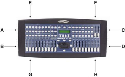
Remove the 4 screws (A, B, C, D) on the side and the 4 screws (E, F, G, H) on the top and bottom. Now you can mount your Light Desk Pro 136 in a 19" rack.
